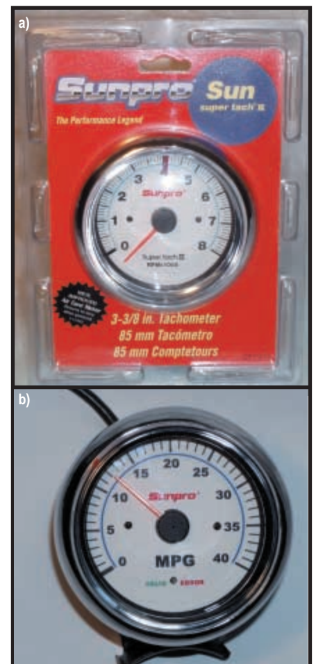
Photo 1—These are before (a) and after (b) photos of my off-the-shelf electronic tachometer from the local auto parts store. I replaced the stock face with my own in order to display miles per gallon. I also added a red/green LED to indicate how well the meter is working.
